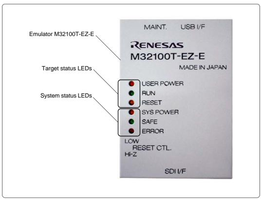
Figure 2.2 Name of each part on the upper panel
